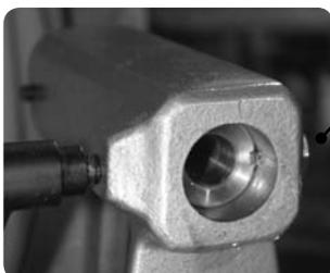
**Note.** Do not adjust the screws at the side of the tailstock as these are factory set.
